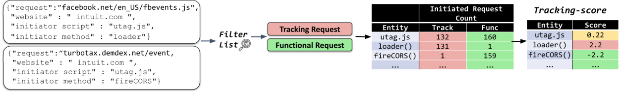
Figure 4.2: Steps for localizing tracking and functional JS code using Spectra-based fault localization. ❶ shows the two network requests on intuit.com . Filter lists are used to label requests in ❷. Spectra-based fault localization is used to classify resources based on participation, as shown in ❸ and ❹.
