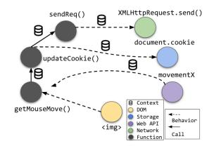
Figure 5.6: A simplified NoT.JS's graph on mouse movement tracking.
