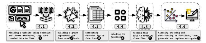
Figure 5.3: NoT.JS pipeline: **1** Crawl sites, save data; **2** Create JS function graph; **3** Extract features and **3** label it; **5** Train classifier; **5** Classify tracking/non-tracking JS functions, and create surrogates.
